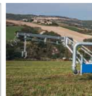
Bandiera porta aspirazione Arm-holder to lift up the suction pipe Bras pour soulever le tuyau d'aspiration
