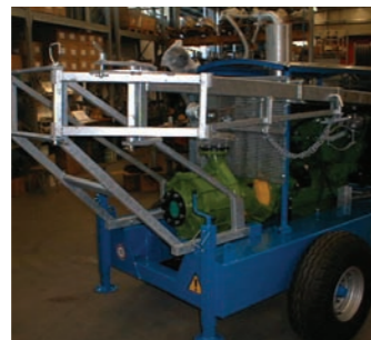
Braccio porta aspirazione idraulico Hydraulic Arm-holder to lift up the suction Bras hydraulique pour soulever le tuyau d'aspiration
